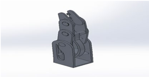
Figure 2: A 3D FEA model of a single finger
