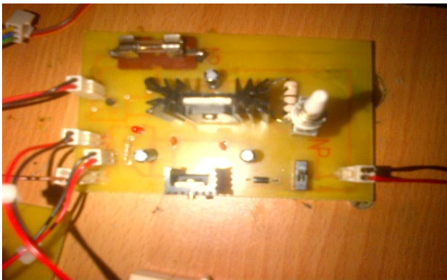
Figure 5: Power distribution circuit connection
