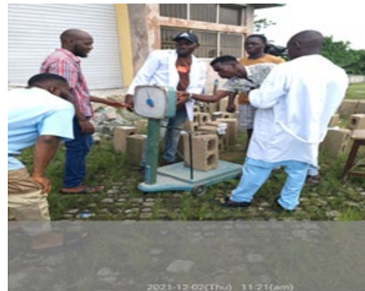
Figure 3: Team members taking mass readings of block specimens
