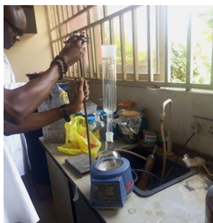
Figure 3: Setting up Soxhlet extraction apparatus
