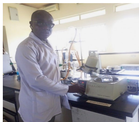
Figure 5: Rotary evaporator for oil separation
