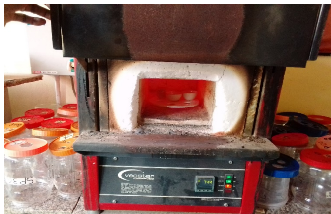
Fig 5: Specimens inside Heat Treatment Furnace
