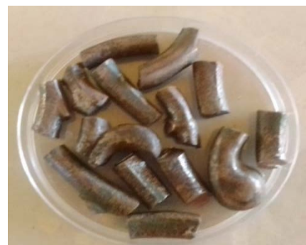
Fig 1: Sample of Cast Iron
