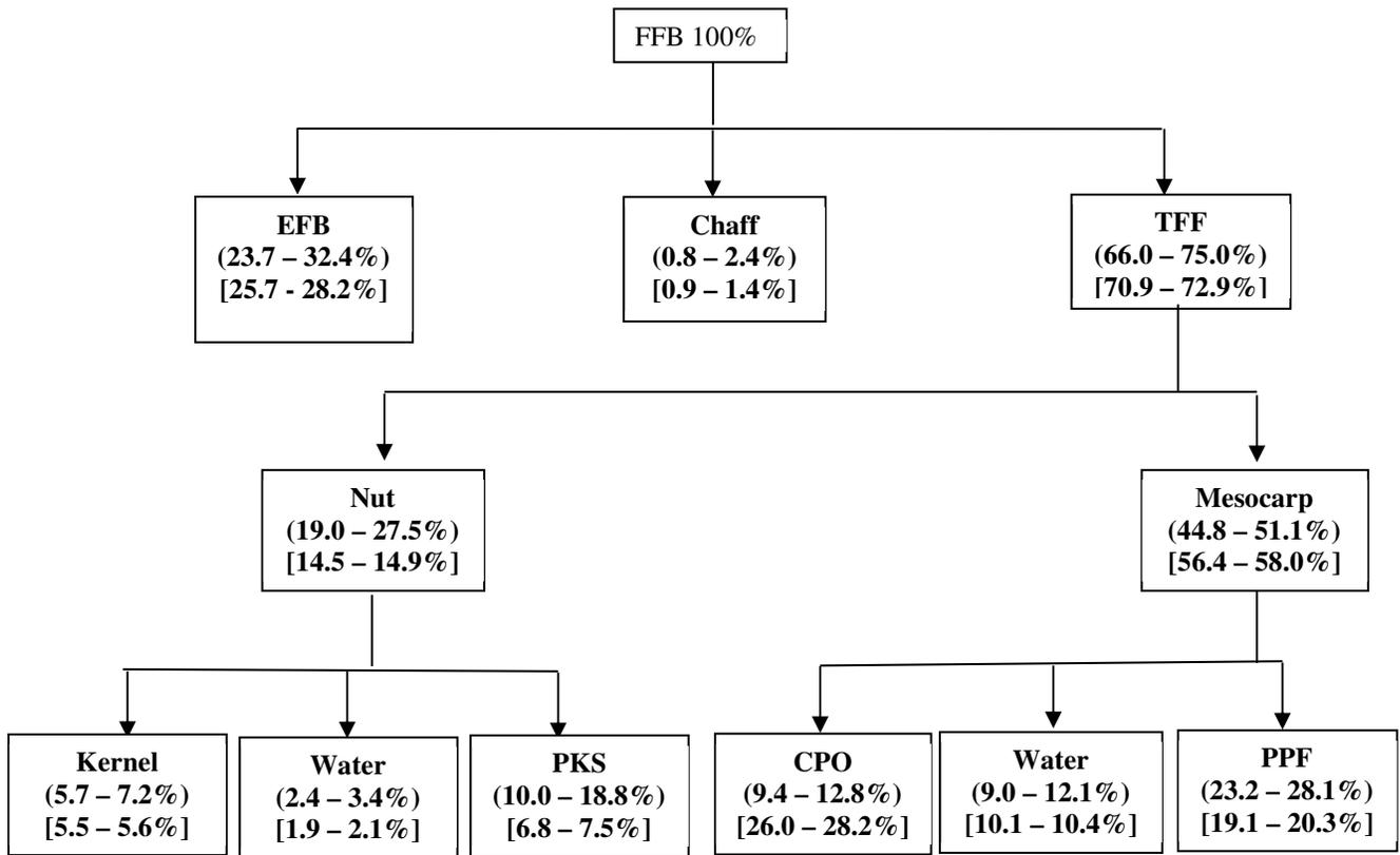
Fig. 15: Material-mass balance of FFB processed by small holders in Nigeria (Ohimain et al 2013f). Figures in bracket are the percentage of the different fraction of FFB: ( ) = *Dura* variety; [ ] = *Tenera* variety.
