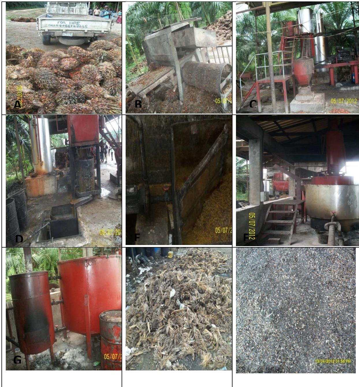
Plate 25: Semi-mechanized oil palm processing; [A] FFB reception [B] Stripper, [C] sterilization/boiling, [D] Digestion and oil extraction zone [E] Clarification zone [F] dryer, [G] Storage of CPO
