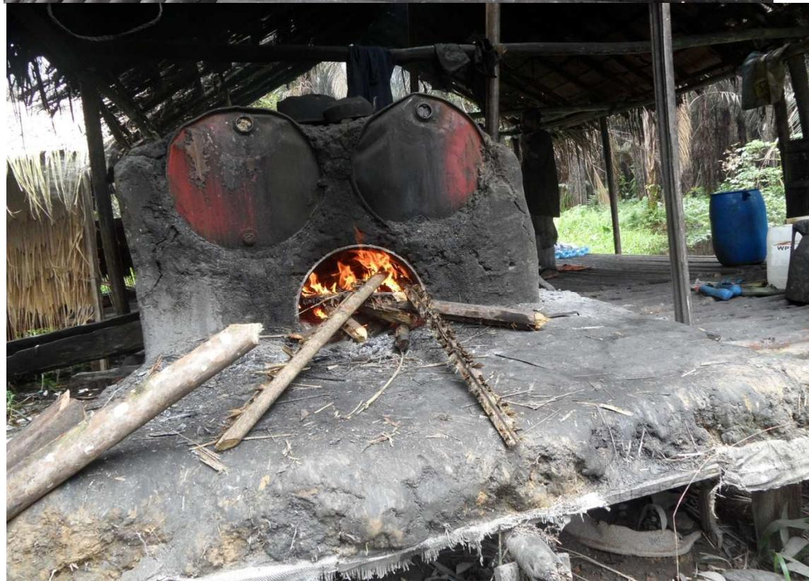
**Fig. 28: Rudimentary ethanol distillation equipment used in the Niger Delta**
