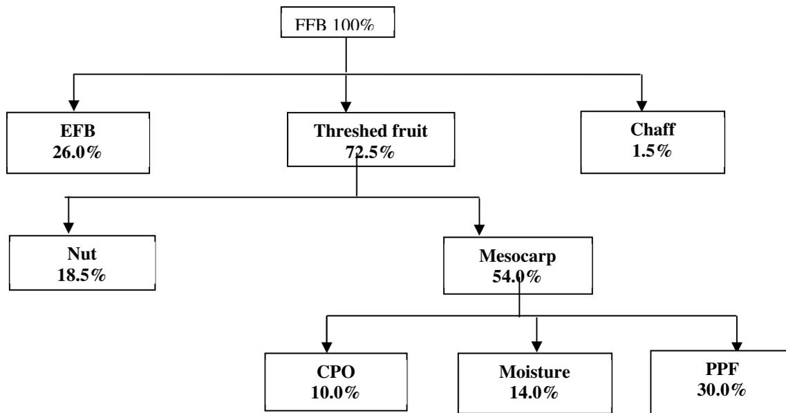
Figure 16: Material mass balance of semi-mechanized oil palm processing in Bayelsa state
