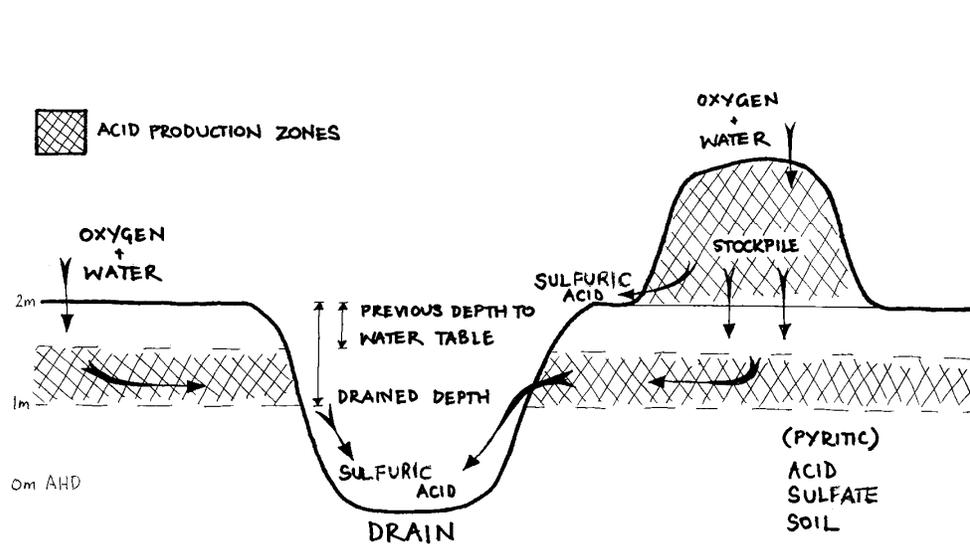
Fig 3: Microbial oxidation of pyrite causing the release of sulphuric acid (Smith *et al.*, 1995)
