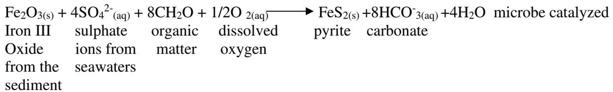
Following the exposure and abandonment of sulphidic dredged materials, acidic drainage results from the interactions of sulphide minerals (pyrite) with oxygen, water, and bacteria (*Acidithiobacillus* sp). The overall stoichiometric reaction describing the oxidation of pyrite is summarized as follows:
