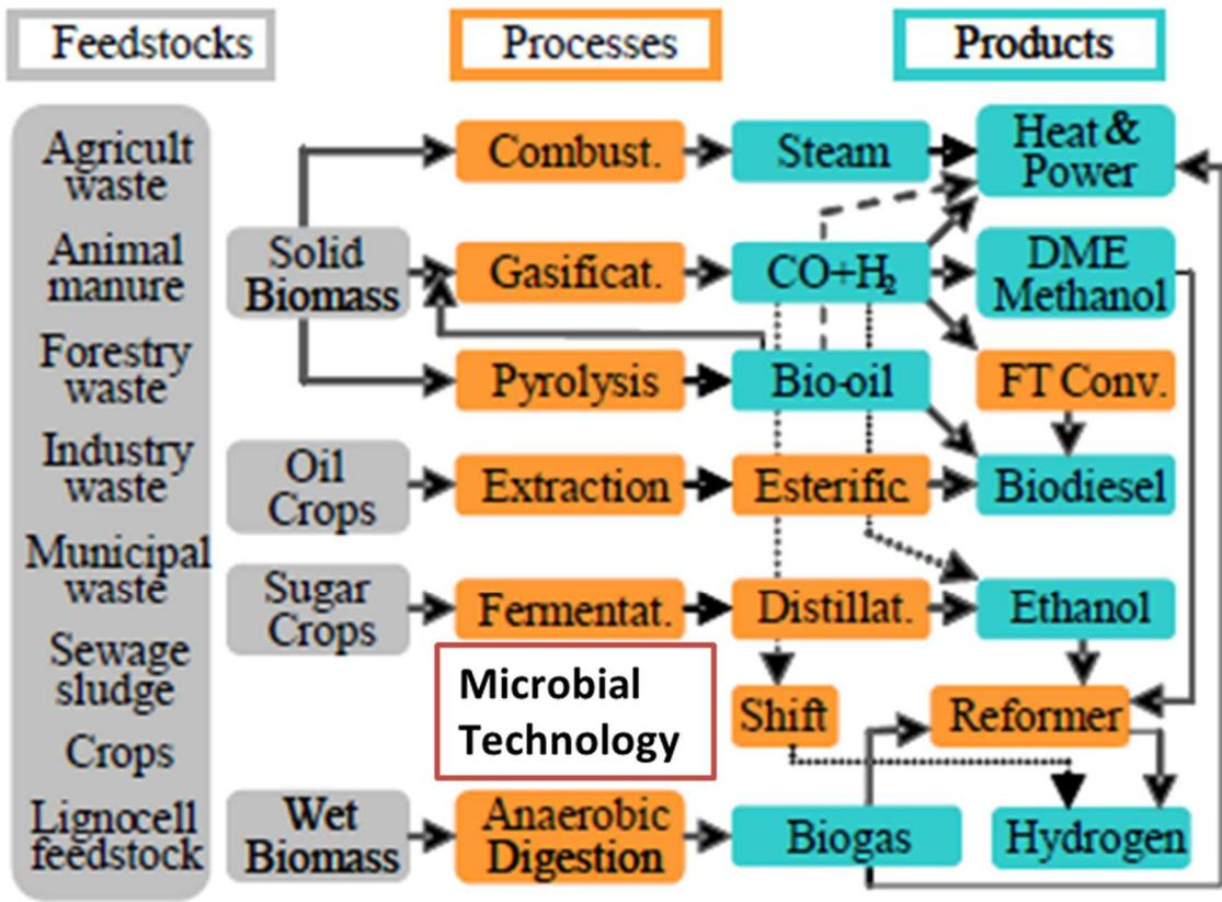
Fig. 7. processes for the conversion of waste biomass to various energy carriers
