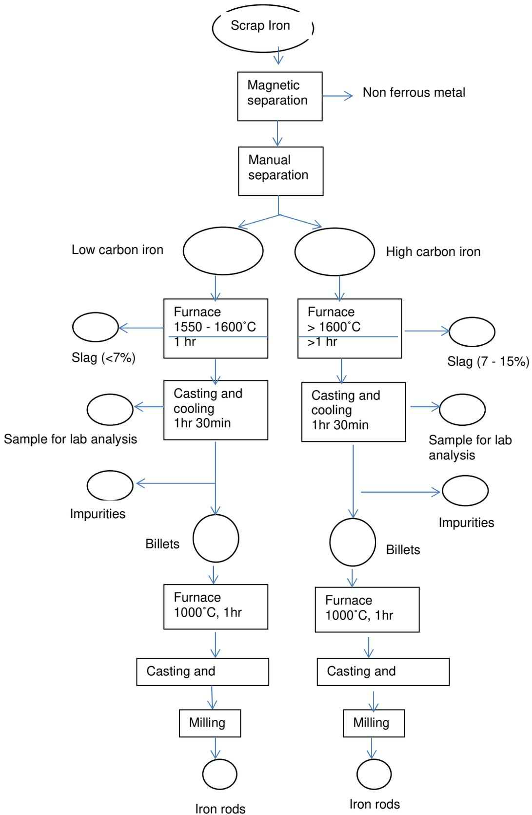
Fig. 26: Scrap iron and steel recycling in Nigeria (Ohimain and Jenakumo 2013)
