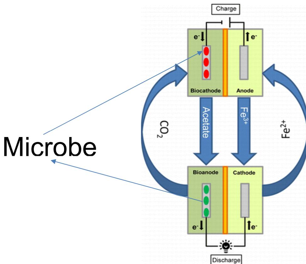
Figure 13: Microbial batteries (modified from Molenaar, et al. 2016)
