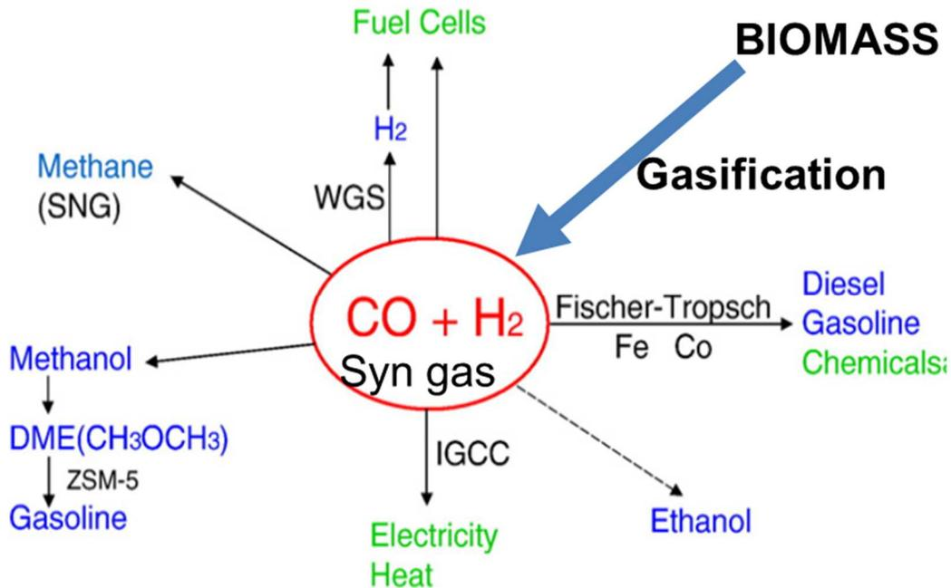
Fig 8: Commercially available fuel products from syngas produced through biomass gasification (modified from Zhang, 2010). WGS= water gas shift; IGCC= integrated gasification combined cycle
