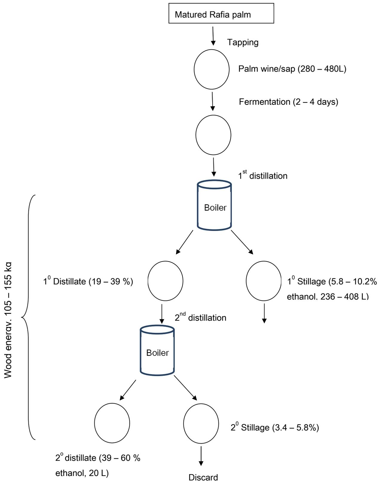
**Fig 19: Batch process for the traditional fermentation and distillation of raffia palm sap for ethanol production**
