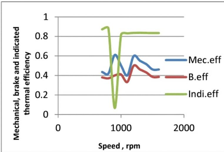
**Fig 2.6:** Graph of mechanical brake and Indicated thermal efficiencies against speed.
