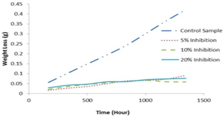
**Fig 5.1:** Weight loss versus time for sample in the corrosive medium with 100% of inhibitor
