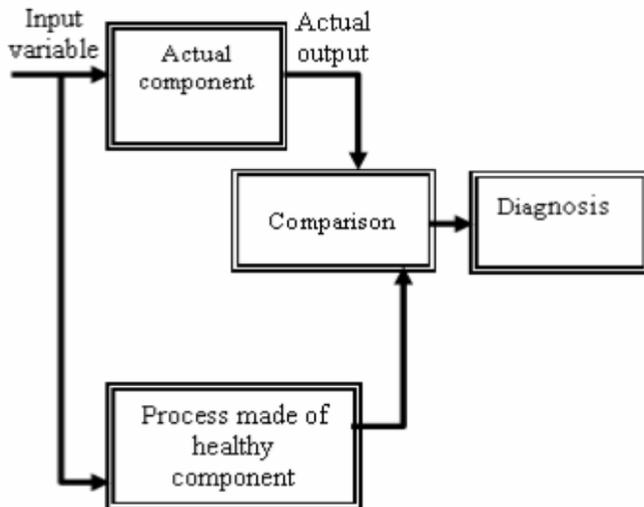
Fig. 2.5: Component model for monitoring and diagnosis.
